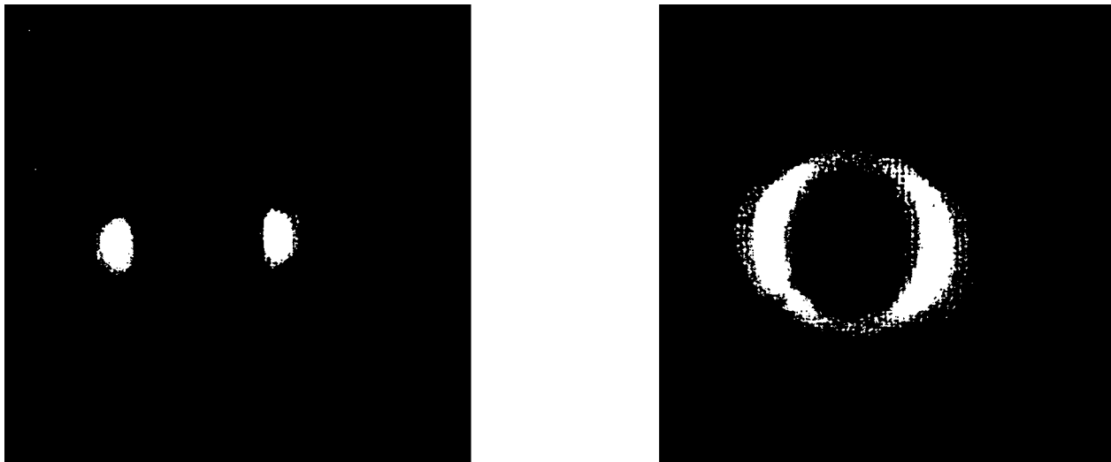
Figure 6 WAXS pattern of Vectra A950 obtained from sheet I (surface of the sample) and from sheet III (center of sample).
